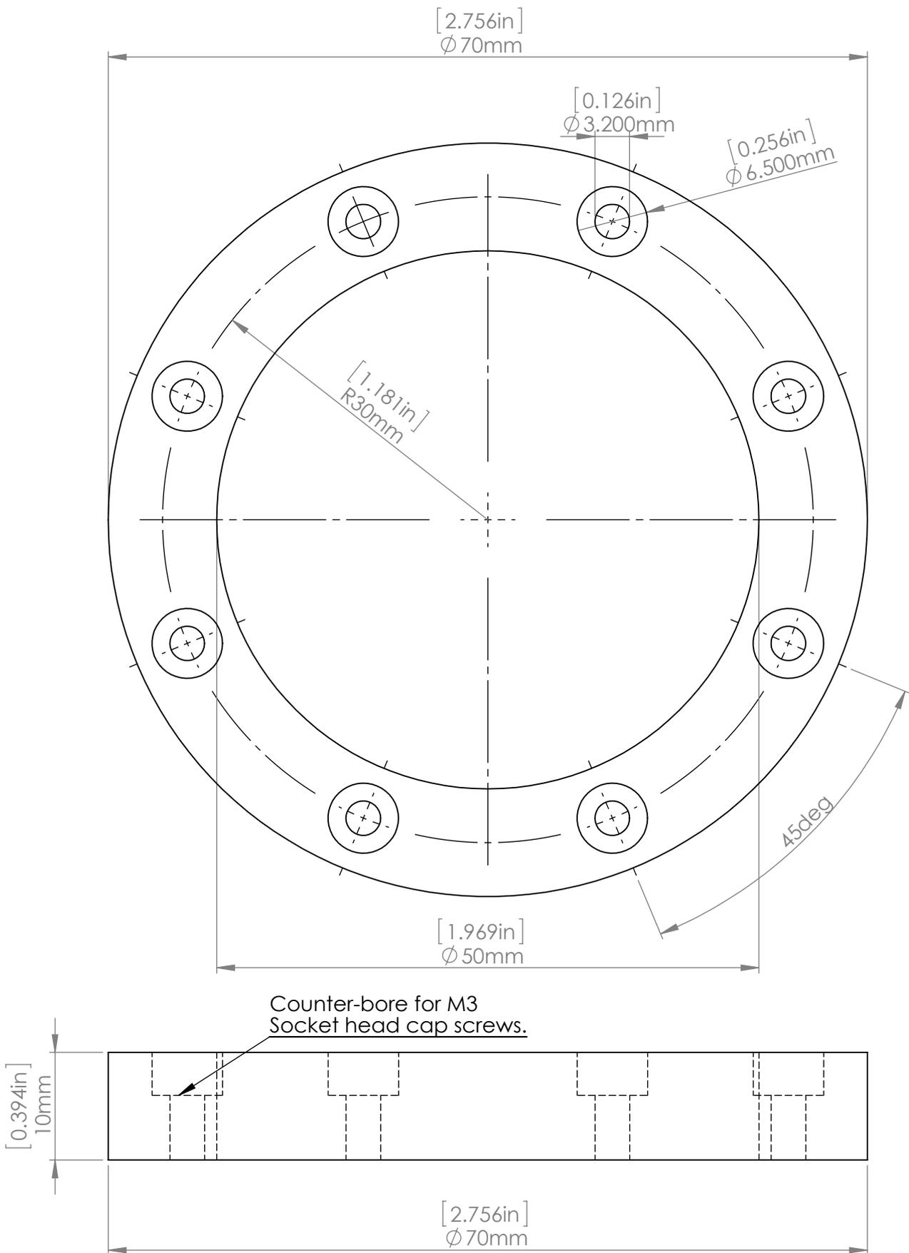
VIEW: TOP, SIDE NOTES: Attaches to Hub Insert and clamps rubber gasket in place
