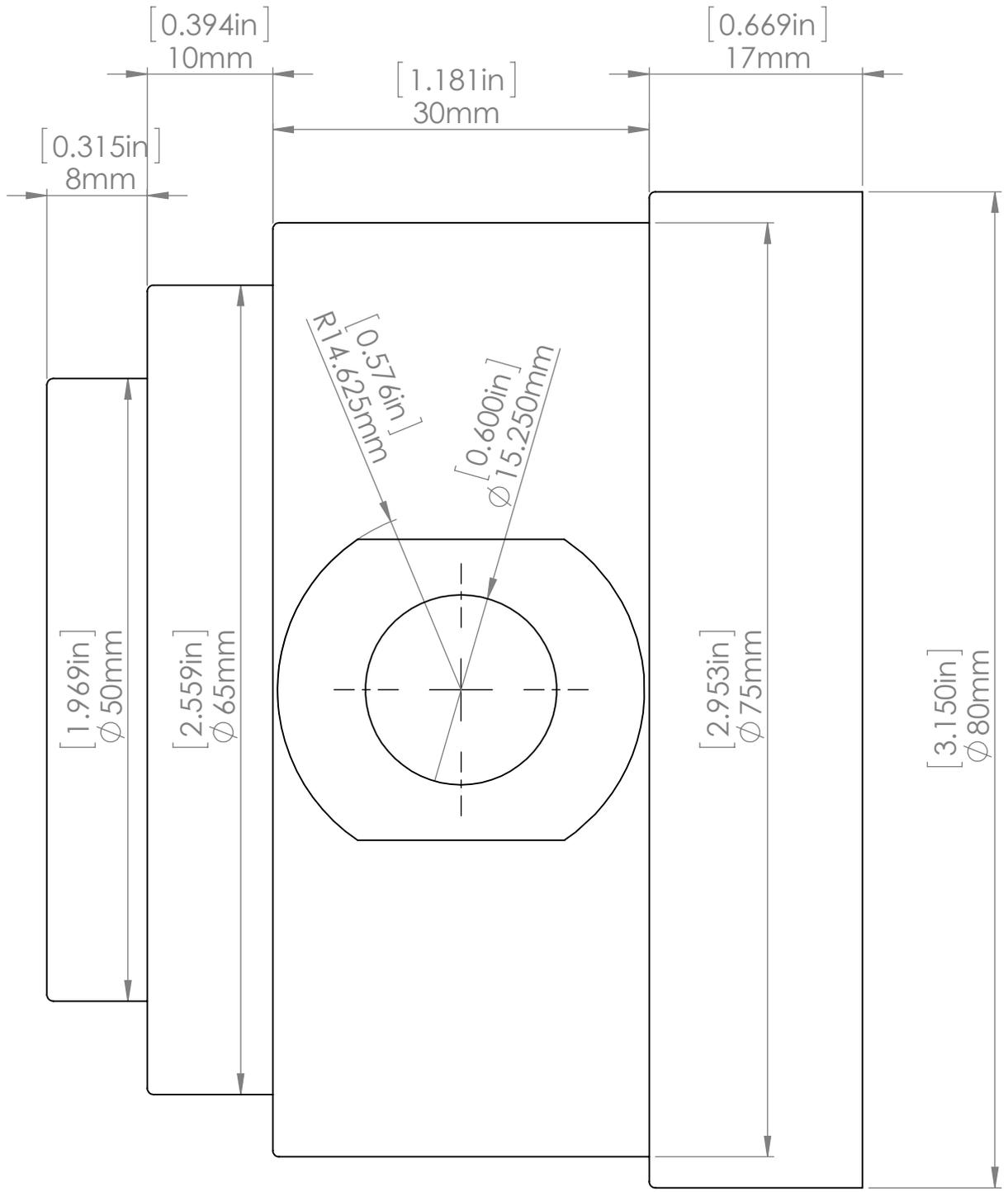
VIEW: TOP NOTES: Top view and exterior dimensions of the hub insert. Interior bore dimensions are shown in other views.
