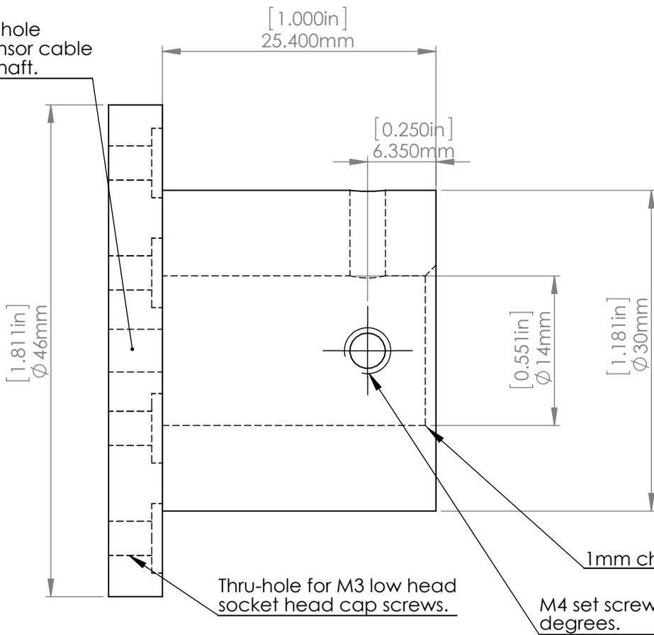
Thru-hole for M3 low head socket head cap screws.
