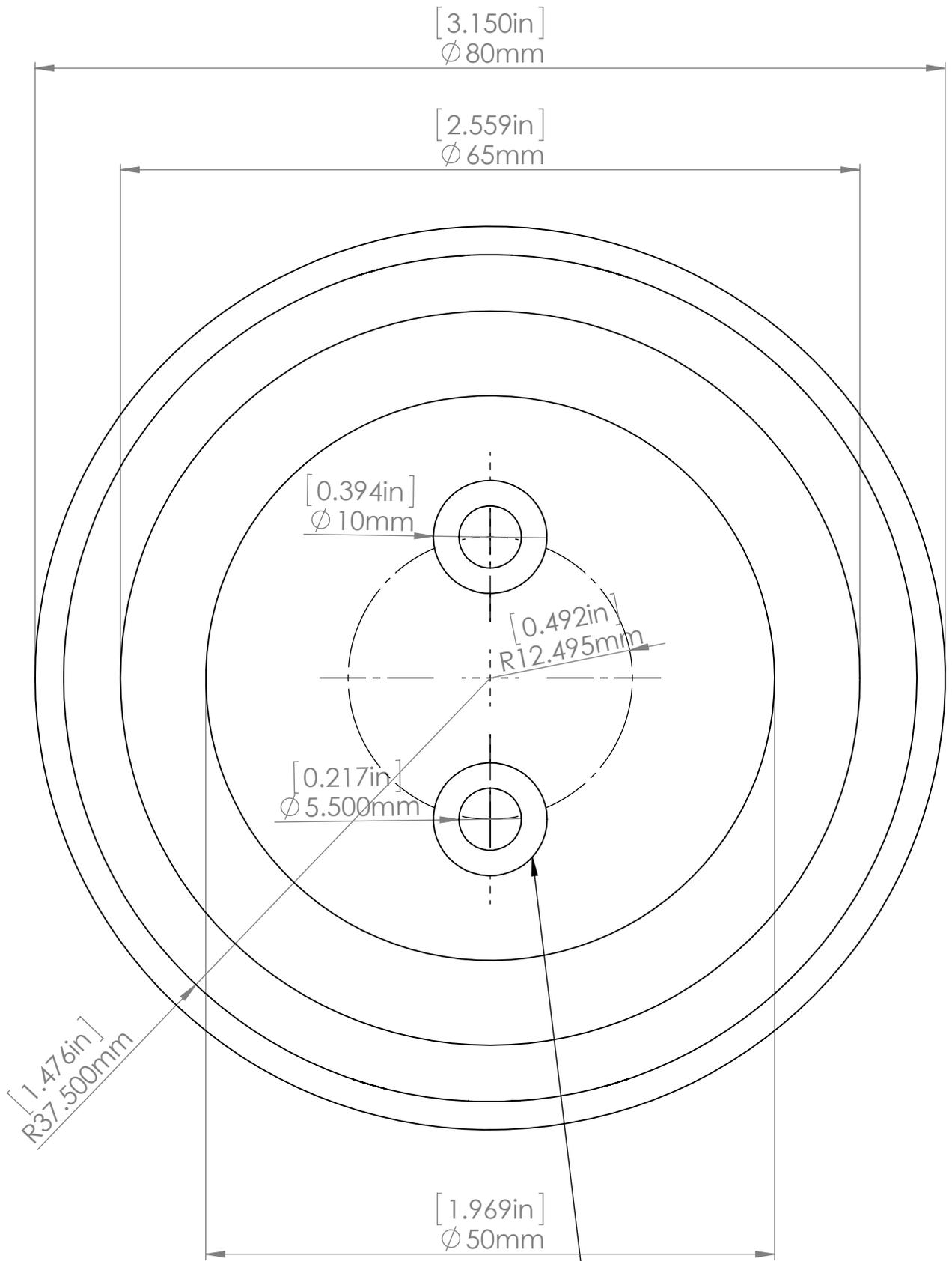
Counter-bore for M5x0.8 socket head capscrews for mounting torquesensor
